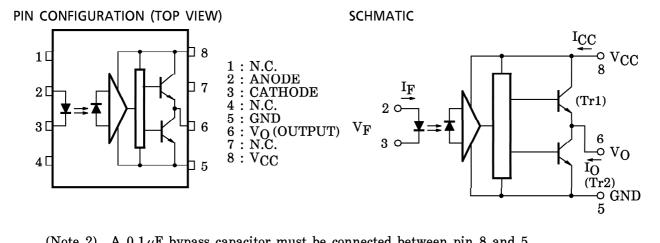
(Note 2) A  $0.1\mu\mathrm{F}$  bypass capacitor must be connected between pin 8 and 5.
